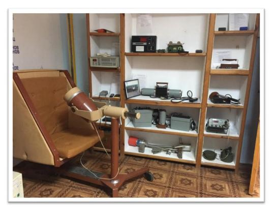
On the left side of the photo, there is a machine looks like a chair and cylinder. This is an old body counter for measuring internal exposure. This machine was introduced in 1990, the detection limit is 2-3 Bq/kg.
