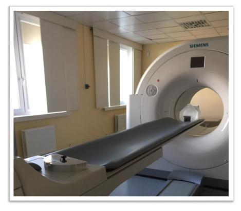
This device is PET-CT. With this device, they can measure the accumulation of nuclides in bone and cardiovascular. Inspection with this device takes about an hour, and it is still plannning stage. It's about just a month since this was introduced.
