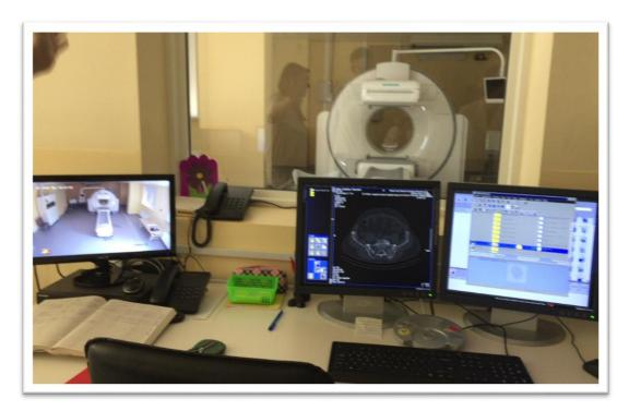
This device is SPECT. With this device, they inspect 10 to 15 patients per day, although it has been just three months since this device introduced. Inspection with this device takes about 30 minutes. Fortunately, we were able to see a patient was undergoing inspection of scintigraphy.
